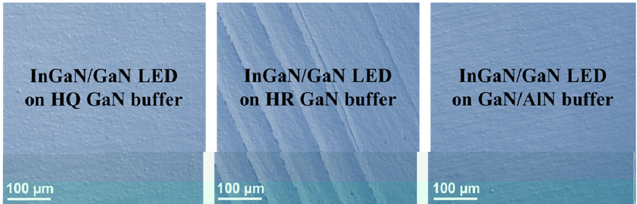
Fig. 9. Surface morphology of InGaN/GaN LEDs on different buffers. (Color figure online)
